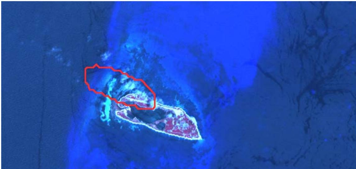
As you can see the coastline is shifted compared to the image. It likely that the *coast\_fill.b* map is not accurate enough for the 15-m ASTER imagery or that the error is introduced in the geo-location performed by HEG.
